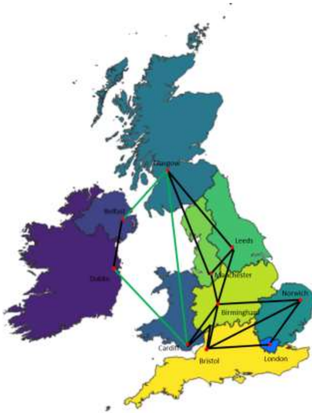
FIGURE 2: SIMPLIFIED HIGH VOLTAGE POWER GRID OF THE UK AND IRELAND: CITIES WITH HIGHEST POPULATION BY SUBREGION HAVE BEEN CHOSEN AS CENTERS OF CONSUMPTION. THE INTERCONNECTION BETWEEN SUBREGIONS WERE ADOPTED FROM [38]. BLACK: HVAC. GREEN: HVDC.
